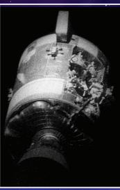
View of the crippled Service Module after separation.
